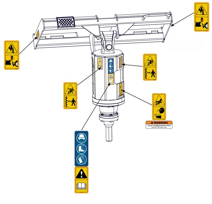
If safety labels have been damaged or removed, new labels must be applied. New safety signs are available from your dealer or contact Reist Industries
